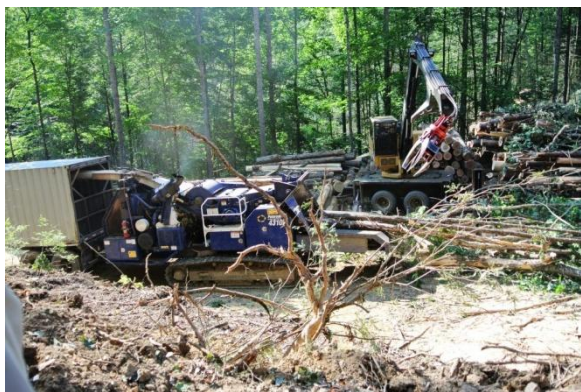
Massive wood chipper turning trash timber into fuel for hybrid power plant. photo by J. Narney
